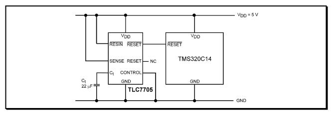
Figure 16. Simple voltage monitoring circuit with the TLC7705
