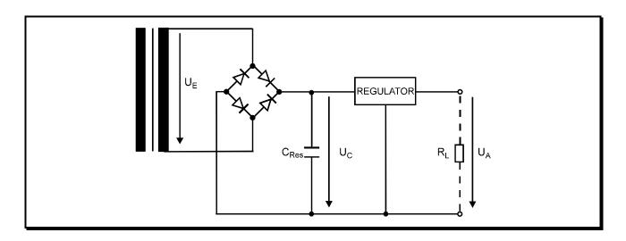
Figure 2. Principle circuit of a Line (Mains) Power Supply  $C_{res}$  t=0 and  $0 < t_1 < T/2$ .
