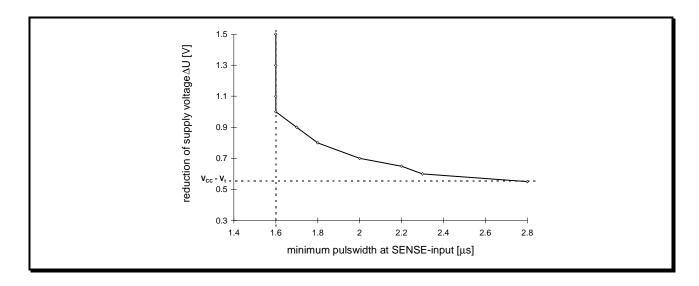
Figure 12. Dependence of the minimum pulse width at the SENSE input on the reduction of the supply voltage (V<sub>DD</sub>=5V)
