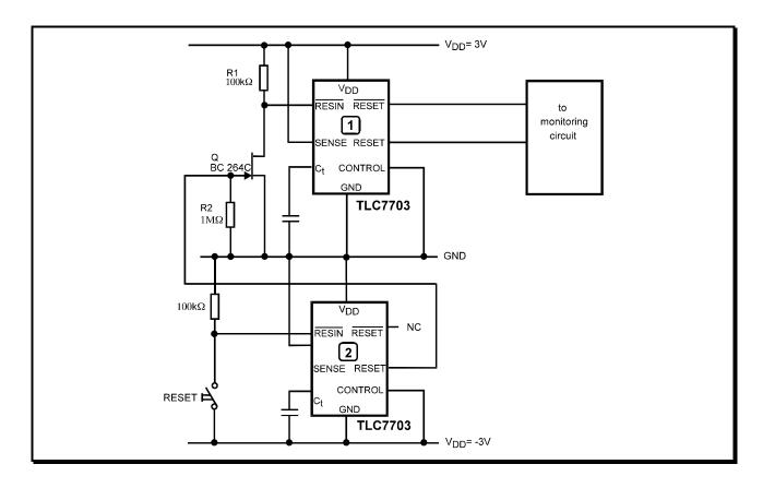
Figure 19. The monitoring of a positive and negative supply voltage
