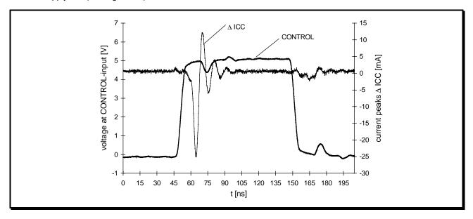
Figure 22. Current peaks on the supply line when switching the RESET output
