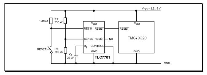
Figure 17. Voltage monitoring circuit for a microcomputer system with the TLC7701
