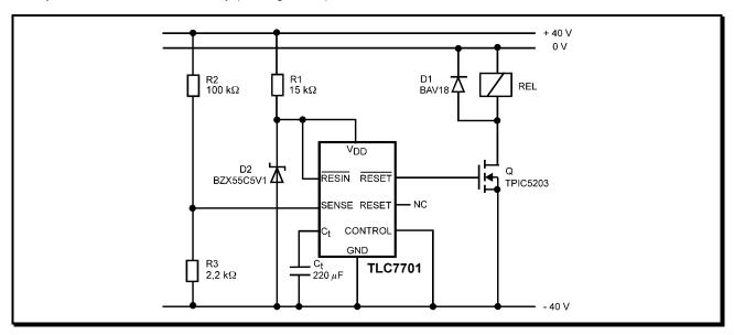
Figure 20. Delay circuit in an audio amplifier
