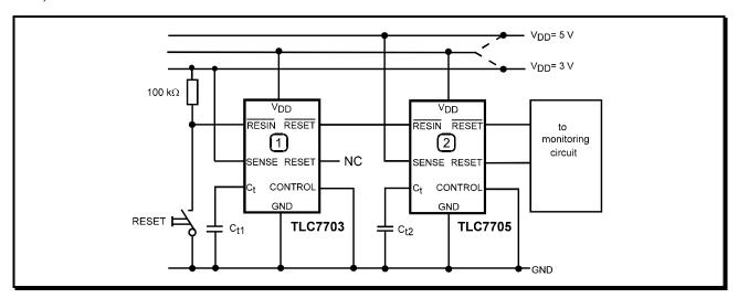
Figure 18. Monitoring of a system with two different supply voltages
