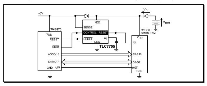
Figure 21. Voltage monitoring in a battery backed memory system
