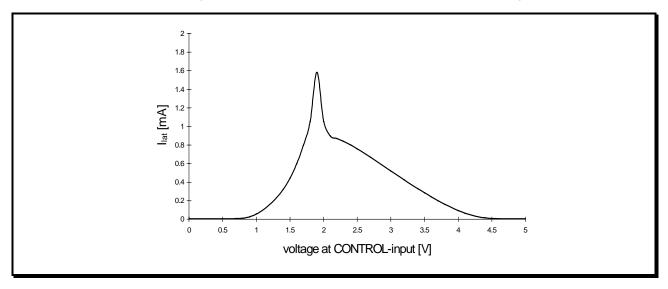
Figure 11. Dependence of the lateral current at the CONTROL input on the input voltage (V<sub>DD</sub>=5V)
