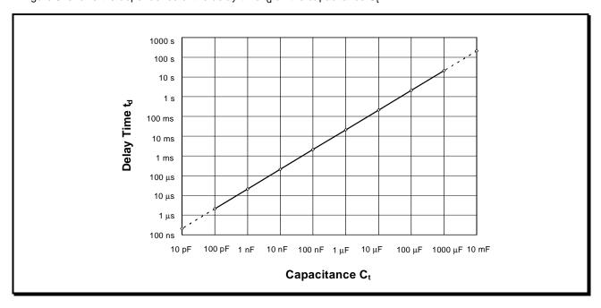
Figure 8. Dependence of the delay time on the capacitance C<sub>t</sub>
