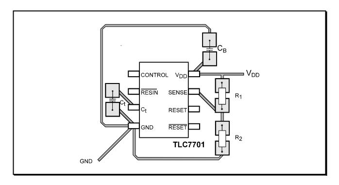
Figure 23. Suggested layout for a circuit board with the TLC7701
