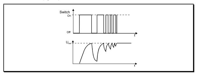
Figure 4. The effect of bouncing switch contacts on the switch-on time of a battery-operated power supply.
