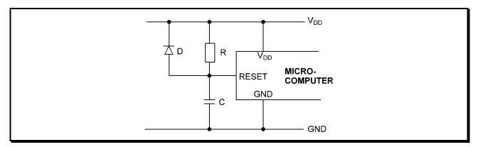
Figure 1. RESET circuit
