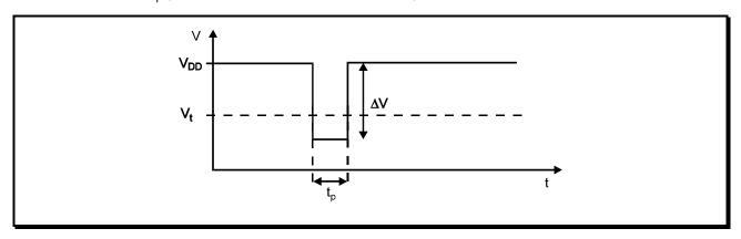
Figure 13. The signal at the SENSE input for determining the minimum pulse width tp
