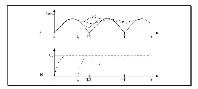
Figure 3. Voltage waveforms in a line operated power supply a) Voltage waveform across the capacitor  $C_{Res}$  when switched-on at a time t=0 and  $0 < t_1 < T/2$ . b) Voltage at the output when switched on at a time  $0 < t_1 < T/2$ .
