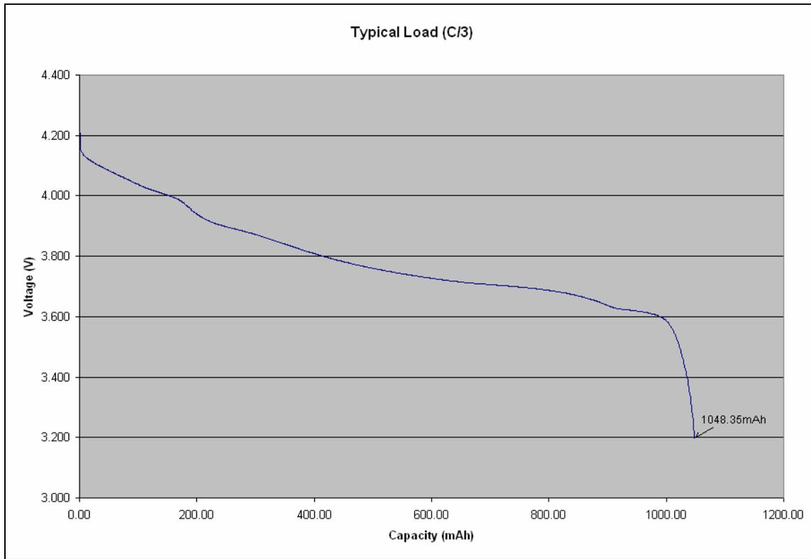
**Figure 1. Determination of Battery Capacity**
