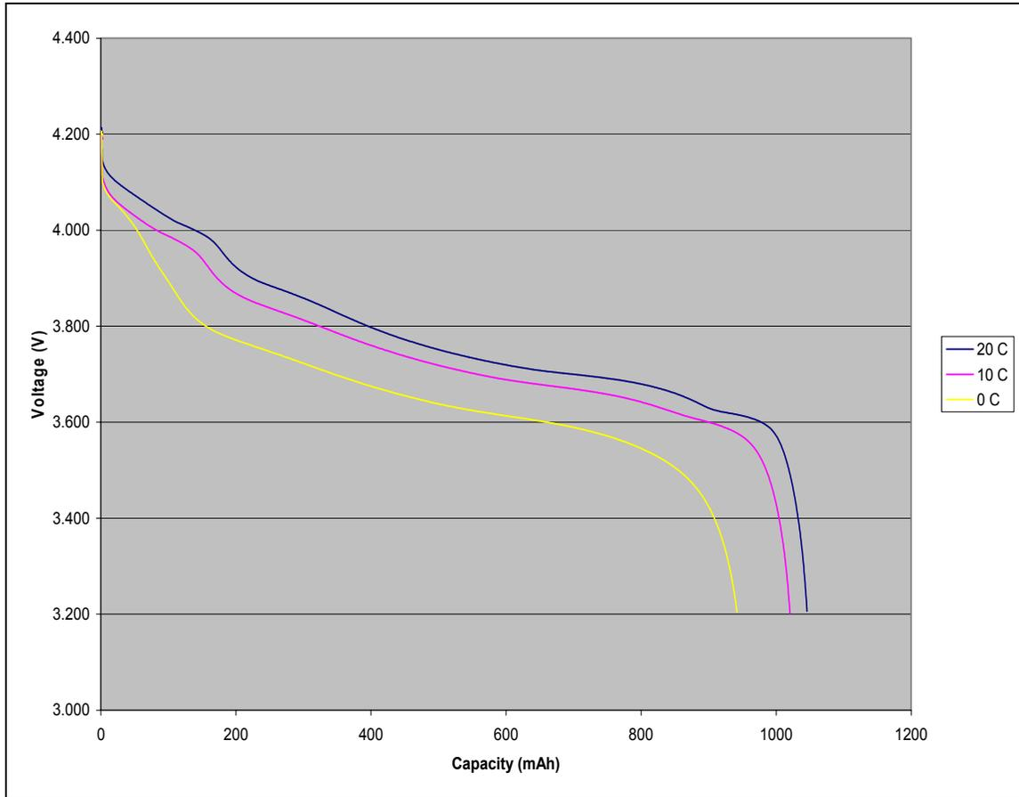
**Figure 6. Discharge Profiles for Different Temperature Rates**
