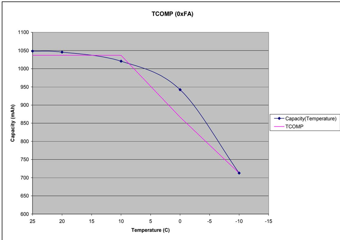
**Figure 7. Curves Used to Determine TCOMP**
