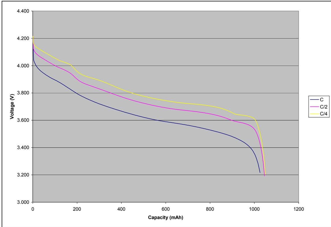
**Figure 4. Discharge Profiles for Different Load Rates**
