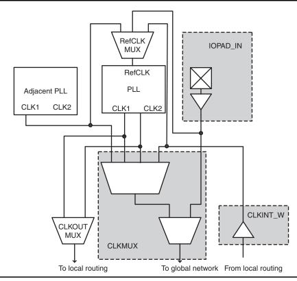
Figure 2 • Clock Network Access Architecture
