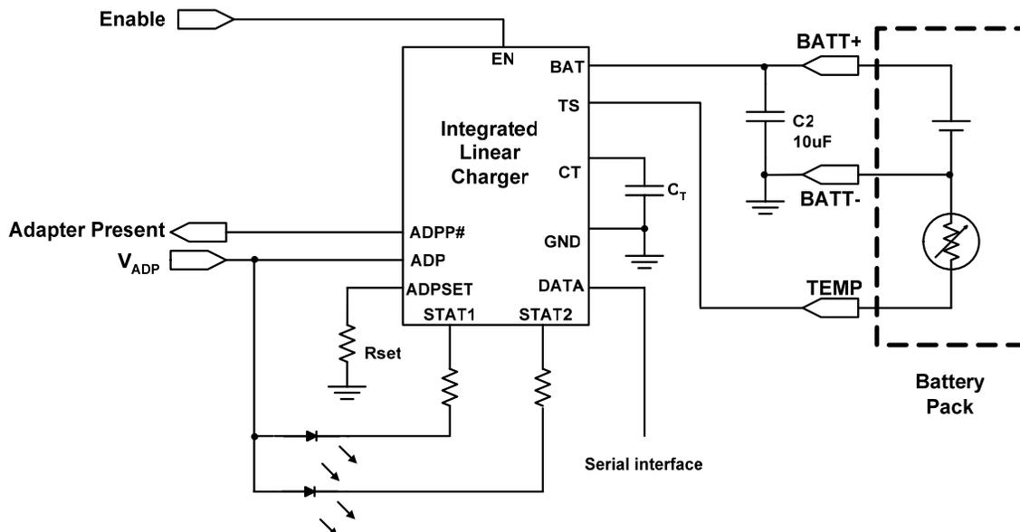
Figure 3: Fully integrated linear Li-Ion battery charger circuit.
