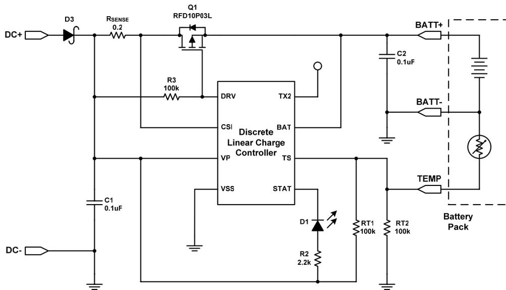
Figure 2: Discrete linear Li-Ion charger circuit.
