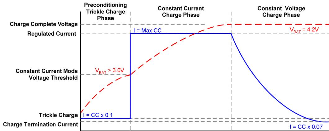
Figure 1: Typical Li-Ion / Li-Poly battery charging profile.
