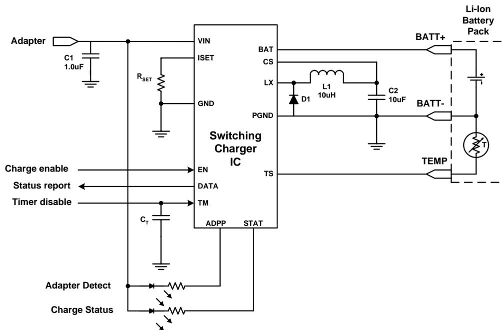
Figure 4: Example DC-DC switching Li-Ion / Li-Poly battery charger circuit.
