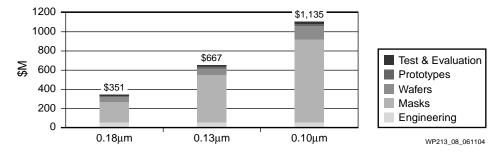
Figure 8: Cost of a custom silicon device re-spin<sup>2</sup>
